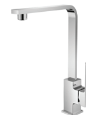
SINK MIXER CHROME S0013688 DZR Brass 25mm Ceramic Cartridge Incl 2x flexipipe connections ISO 9001 & 14001 Balance Pressure System: SAN 102521 Balance Pressure: SANS 10254
