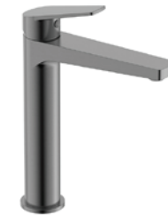
COLD START HIGH BASIN MIXER GRAPHITE S0016516 DZR Brass 35 mm Ceramic Cartridge Incl 2x flexipipe connections ISO 9001 & 14001 Balance Pressure System: SAN 102521 Balance Pressure: SANS 10254
