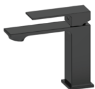
BASIN MIXER POWDER COATED BLACK S0013686 DZR Brass 30mm Ceramic Cartridge Incl 2x flexipipe connections ISO 9001 & 14001 Balance Pressure System: SAN 102521 Balance Pressure: SANS 10254
